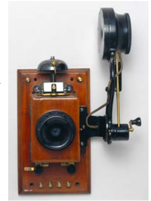
A telephone from 1877 with Edison’s improvements
